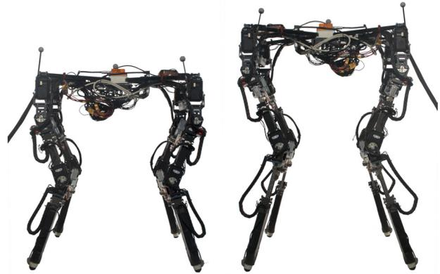
**Figure 1: Our shape-shifting robot, with retracted legs to the left, and extended legs to the right.**
