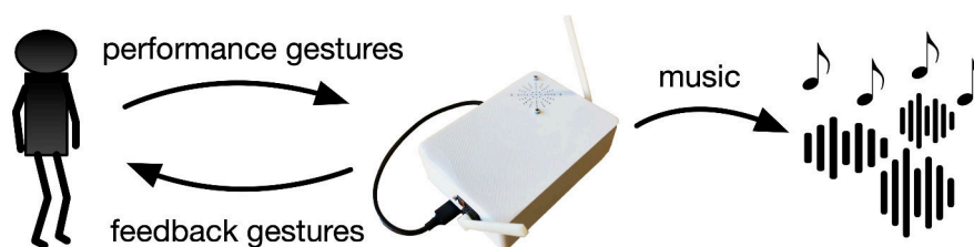
Figure 2: Typical musical instruments translate physical gestures into musical sounds. A predictive instrument can guess future gestures and use this knowledge to provide continuous sonic output and physical feedback to the performer.
