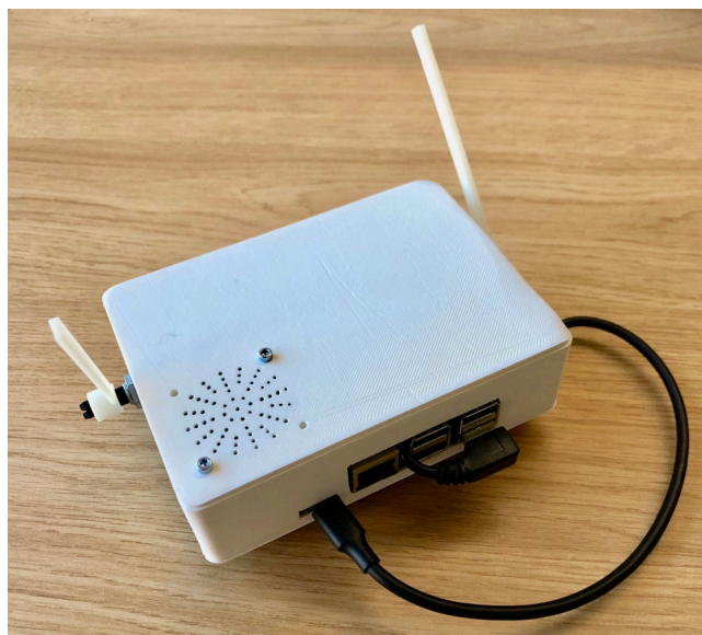
Figure 1: The Embodied Music Prediction Interface (EMPI) prototype. The system includes a lever for a performer’s physical input (left side) and a motor-controlled lever for physical output, a speaker, and Raspberry Pi. This system represents a minimum set of inputs and outputs to experiment with embodied predictive interaction. A demonstration video can be viewed at https://doi.org/10.5281/zenodo.3521178
